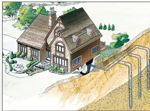
Example of a vertical, closed-loop system.
